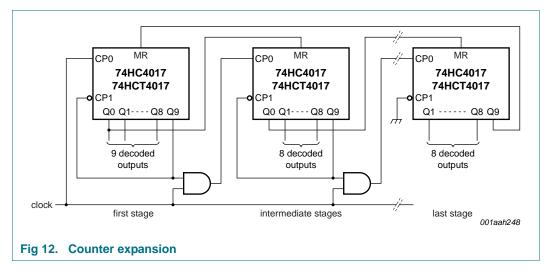
**Remark:** It is essential not to enable the counter on  $\overline{CP1}$  when CP0 is HIGH, or on CP0 when  $\overline{CP1}$  is LOW, as this would cause an extra count.
