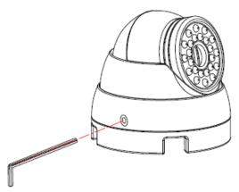
2. Unscrew the Outer Housing by twisting it counterclockwise and then remove the outer Housing from the Camera Base.
