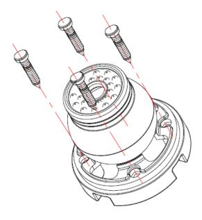
b. If you want to wire the cables through the wall, attach and thenscrew the Camera Base to the ceiling / wall. Attach the CameraBody to the Camera Base.
