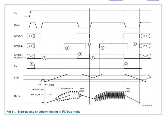
Table 20. Start-up and shutdown timing in I<sup>2</sup>C-bus mode
