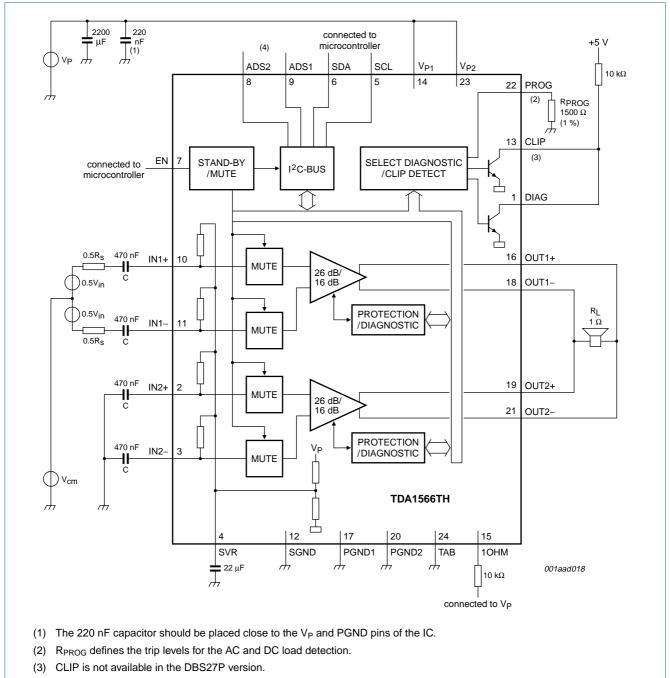
(4) I<sup>2</sup>C-bus mode is selected with ADS1 open. ADS2 is not available in DBS27P version.
