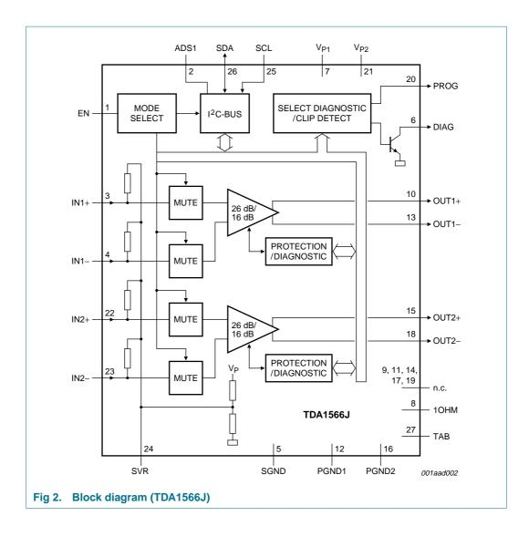
I<sup>2</sup>C-bus controlled dual channel/single channel amplifier
