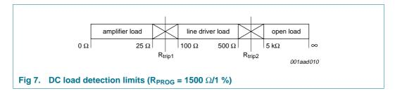
The relation between  $R_{PROG}$ ,  $R_{trip1}$  and  $R_{trip2}$  is approximated by (valid for  $R_{PROG}$  should be between 1.2  $k\Omega$  and 4  $k\Omega$ ):
