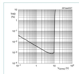
$R_L$  = 100  $\Omega$ ; 80 kHz measurement filter; f = 1 kHz.
