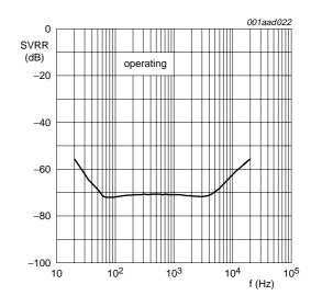
$R_s = 1 \text{ k}\Omega$ ;  $C_{SVR} = 10 \mu\text{F}$ .
