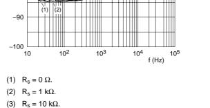
Fig 17. Channel separation as a function of frequency
