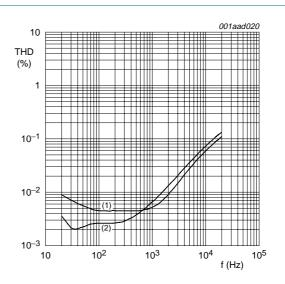
$R_L = 4 \Omega$ ; 80 kHz measurement filter.
