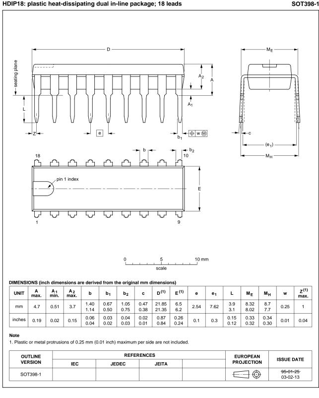
HDIP18: plastic heat-dissipating dual in-line package; 18 leads
