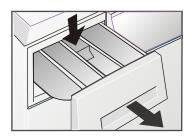
Pull out the detergent dispenser up to the end stop, press down the hollow on the insert and remove the detergent dispenser completely.
