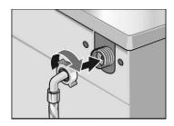
Connect the water supply hose:To the back of the washing machine, and...
