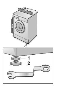
All four appliance feet must be firmly on the ground. The washing machine must not wobble.
