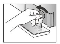
Carefully remove the pump cap.But don't fully remove it and allow a little more residual water flow into the suitable container.
