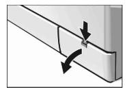
This is necessary if the washing solution can not be completely drained. The pump is blocked by either loose debris or fluff which accumulates if fluff-giving fabrics are washed at high temperature.
