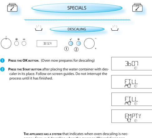
essary. Carry out descaling when the message "Descale" appears on the display. Before carrying out descaling, make sure you have enough descaling liquid available. We recommend that you use "Wpro active'clean" descaler suitable for coffee / espresso machines and kettles.
