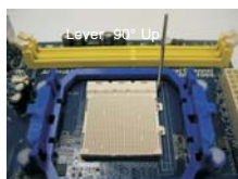
STEP 1: Lift Up The Socket Lever
