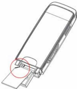
**The SIM slot is located above the USB connector**
