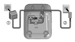
First connect the mains unit (230 V) to power cord ① and then connect the phone jack to phone cord ②, as shown above. Place the cords in the cord recesses. The two cords must be plugged in at all times.
