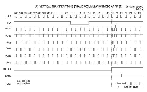
\* Do not use the frame signals immediately after field accumulation mode is transferred to frame accumulation mode.
