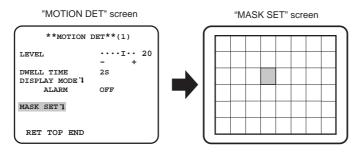
In the masked area, no alarm will be issued even if a moving object is detected. The masked area is set in the same way as the masked area setting in Light quantity control method selection. (respage 11)
