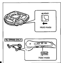
This function causes the unit to ignore short, accidental button presses. (The disc lid can still be opened and closed.)
