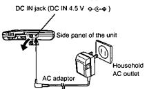
Turn the unit off before connecting or disconnecting the AC adaptor.
