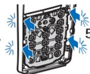
6. To replace the front cover (6), press it gently on the phone, beginning from the bottom.
