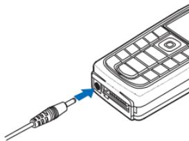
The charging time depends on the charger and the battery used. For example, charging a BL-5C battery with the ACP-12 charger takes approximately 1 hour and 30 minutes while the phone is in the standby mode.
