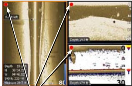
Red circle indicates sonar log is being recorded; All Channels are being logged in this example
