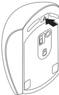
2. Insert the two batteries according to the polarity indicators in the mouse.
