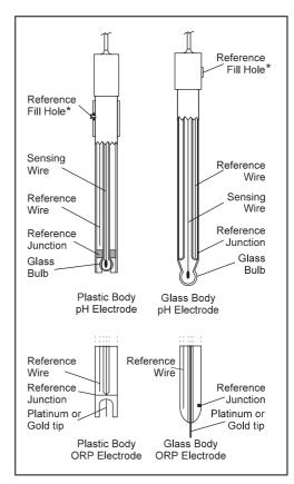
\* Only for refillable electrodes; must be open while measuring.
