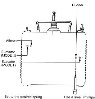
strength by turning the screw of each stick.
