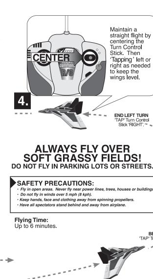
To end turn 'TAP' the Turn Control Stick to the RIGHT just enough to level the wings and fly straight. 'TAP' the Turn Control Stick LEFT several times to turn. Fast repeated taps for tight turns, slow repeated taps for wide turns. (It's easier to start with left turns when first learning).
