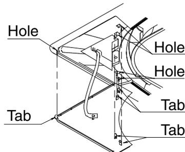
Attach by inserting the five tabs on the corner section decoration cover into the holes on the decoration panel.
