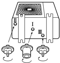
Be sure to insert sockets and caps into their proper drain holes to prevent water leakage.
