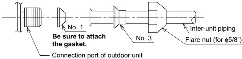
(2) Connecting a pipe of  $\phi 3/8''$  to a gas pipe connection port for  $\phi 5/8''$ :
