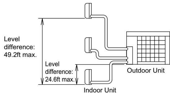
If the outdoor unit is positioned lower than one or more of the indoor units.
