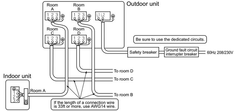
Use AWG 16 or AWG 14 wire for the power supply and interconnecting wires.
