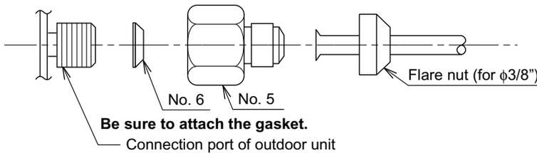
(3) Connecting a pipe of  $\phi 3/8''$  to a gas pipe connection port for  $\phi 1/2''$ :
