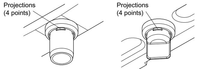
3. Connect vinyl hose on the market (internal diameter of 1 inch) to drain socket (A). (If the house is too long and hangs down, fix it carefully to prevent the kinks.)
