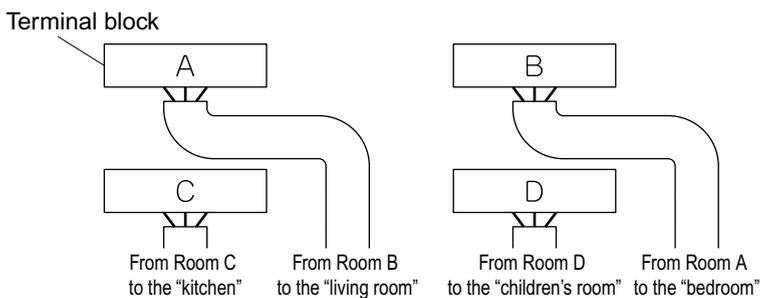
\* The figure at left shows branch wiring.
