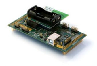
The RZ541 Packet Sniffer Kit is the ideal platform for analyzing 802.15.4(TM) and ZigBee wireless networks. Included is the basic edition of the Sensor Network Analyzer software from Daintree Networks which enables visualisation, measurement, and analysis of large networks.
