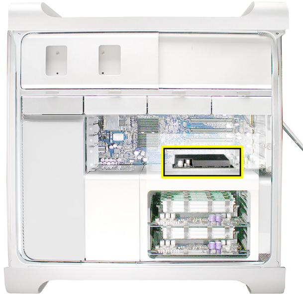
3. Loosen the two captive screws that secure the PCI bracket to the enclosure and remove the bracket.
