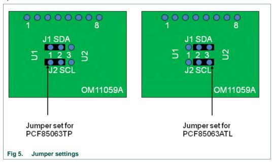
On the market, there are quartzes with different load capacitance  $C_L$ . 12.5 pF is most common, 7 pF offers however lower power consumption. To evaluate the difference, the PCF85063TP is connected to a quartz with  $C_L$ =7 pF and the PCF85063ATL is connected to a quartz with 12.5 pF. Also the  $V_{DD}$  blocking capacitors are mounted (C1, C2).
