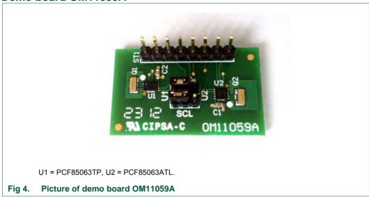
The OM11059A allows to easily demonstrate the operation of the PCF85063x with I<sup>2</sup>C-bus interface. No need to solder the tiny package to a breadboard 100 mil connector for straight forward connections.
