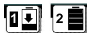
Batteries in wells 1 and 2; battery in well 1 discharged, battery in well 2 is fully charged, not in use
