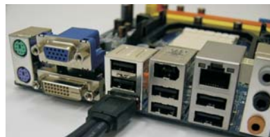
Connect the other end of the eSATAII device cable to eSATAII port of the I/O shield
