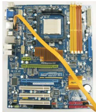
Connect the SATA data cable to the eSATAII connector (eSATAII_TOP)
