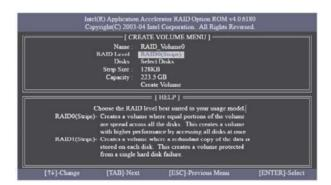
Use the up or down arrow keys to select your desired **RAID** Level. You may select RAID 0 (Stripe), RAID 1 (Mirror), RAID 5 or RAID 10 for your RAID level. Press <Enter>, and then you can select **Strip Size**.
