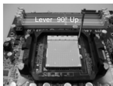
STEP 1: Lift Up The Socket Lever
