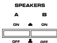
\* If you use two front speaker systems, press both the A and B switches.
