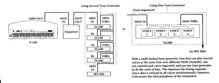
In this connection example, the sequencer is used for recording and playback, while four different MIDI instruments are connected in "daisy chain" fashion. The effect unit tagged onto the end of the chain is controlled over the Extra MIDI A Path.
