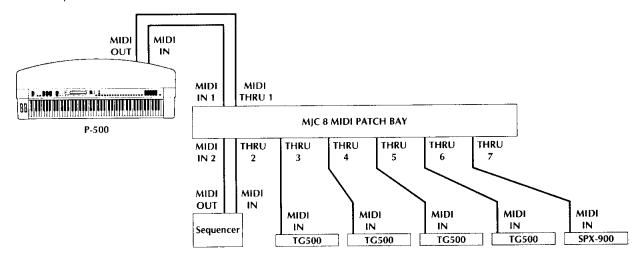
In a variation of the extended MIDI system above, a MIDI patch bay (such as the Yamaha MJC8) is used to "direct traffic" for the complex MIDI signal routings.
