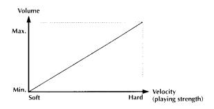
The P-500, however, provides a total of twenty different Velocity Curves. This allows you to tailor the keyboard response to fit the way you play, as well as set up separate curves for the various Paths in order to selectively and gradually bring in different sounds depending on how softly or strongly you play.
