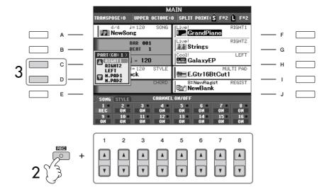
3 Use the [C]/[D] buttons to select the desired part for the channel to be recorded.
