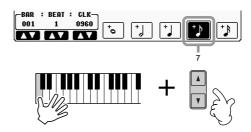
While holding the C3 and E3 keys on the keyboard, press the [7▲▼]
