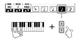
While holding the C3, E3, G3 and C4 keys on the keyboard, press the [7 ▲ ▼] button, and successively press the [5 ▲ ▼] button.
