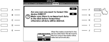
In this example, press the [F] (YES) button to start formatting the USB storage device (USB flash memory, floppy disk, etc.).
