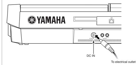
4 Connect the other end (normal AC plug) to the nearest electrical outlet.
