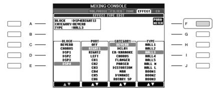
10 If you have selected one of the DSP 2-4 effect blocks in step 5: You can edit its standard parameters as well as its variation parameter. To select the standard type of parameters, press the [B] button. To select its variation parameter, press the [E] button.
