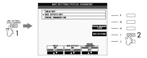
Press the [I] (MIC SETTING) button to call up the MICROPHONE SETTING display.
