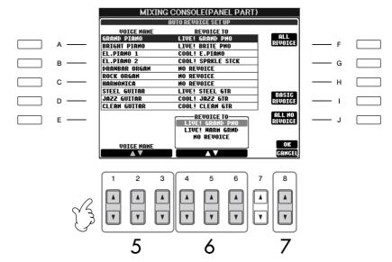
6 Use the [4 ▲ ▼]-[6 ▲ ▼] buttons to select the Voice for replacing the XG selected in step 5.
