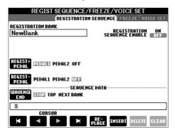
If you intend to use a pedal to switch Registration Memory settings, specify here how the pedal will be used—to advance or to reverse through the sequence.
