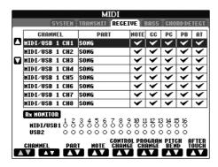
The explanations here apply to the RECEIVE display to be called up in step 4 of the "Basic Operation" on page 204. This determines which parts will receive MIDI data and over which MIDI channels the data will be received.
