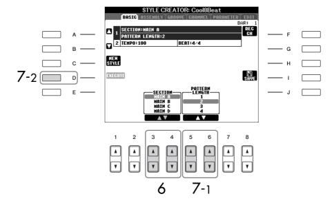
7 Use the [5 ▲ ▼]/[6 ▲ ▼] buttons to determine the length (number of measures) of the selected section.
