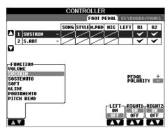
The functions assigned by default to the connected footswitch or foot controller can be changed—for example, letting you use the footswitch to start/stop Style playback, or use the foot controller to produce pitch bends.
