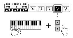
While holding the C3, E3 and G3 keys on the keyboard, press the [7 ▲ ▼] button.
