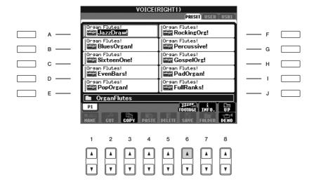
3 Use the TAB [◄][▶] buttons to call up the relevant setting display. For information on the available parameters, see the "Editable Parameters in the VOICE SET [ORGAN FLUTES] displays" on page 104.
