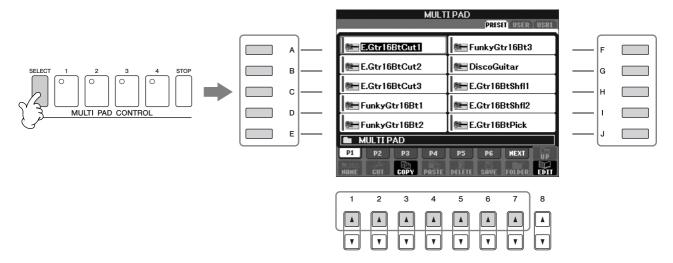
Select pages using the  $[1 \blacktriangle]$ – $[7 \blacktriangle]$  buttons that correspond to "P1, P2..." in the display, then use the [A]–[J] buttons to select the desired bank.
