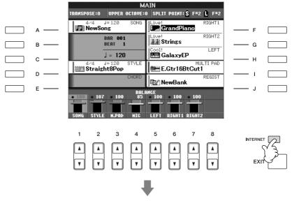
To close the website display and return to the operation display of the instrument, press the [EXIT] button.
