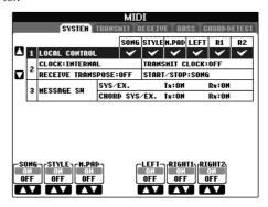
4 Use the TAB [◄][►] buttons to call up the relevant setting display.
