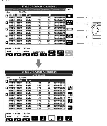
In the EDIT display, you can record notes with absolutely precise timing. This Step Recording procedure is essentially the same as that for Song Recording (page 152), with the exception of the points listed below:
