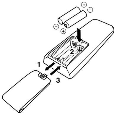
**1** Press the part marked with a
