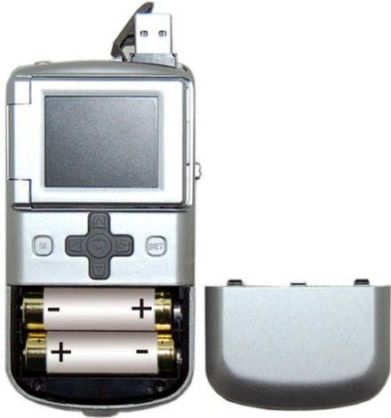
Slide open the battery cover on the back of the camera and install 2 x AA batteries with the correct polarity as illustrated inside the battery compartment. Alkaline batteries recommended.
