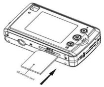
3. Push the card in until you feel and hear it "click" into position. The top of the card should be flushed with the surface of the camera. A icon will appear on the top right of the LCD screen.
