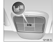
Control indicator ⊌\* for Vauxhall child restraint systems with transponders \*: Vauxhall child restraint systems with transponders can be identified by a sticker - see Fig. 11382 AQ.
