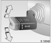
Operating turn signal lights: Right = Stalk all the way up Left = Stalk all the way down Turn signal stalk returns to its original position after use. When steering wheel steering wheel to operate headlight is straightened up, turn signal lights are flash. automatically cancelled.
