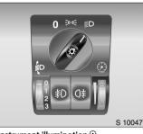
Instrument illumination 2, information display illumination: exterior lights are on: Turn adjustment wheel until desired
