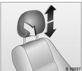
Adjusting head restraint height: Grip headrest at sides, tilt forward, hold and adjust height, engage.
