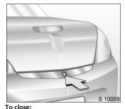
Press and hold the button below the luggage compartment lid until it is completely closed.
