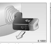
Operating windscreen wash system and headlight wash system \*: Pull stalk towards steering wheel. The wiper swipes for a few strokes.
