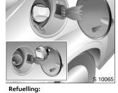
Open tank flap, unscrew fuel filler cap, remove and suspend from tank flap. The fuel tank has a limiting system which
