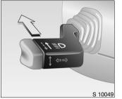
Activating main or dipped beam: Main beam = Move stalk forward Dipped beam = Stalk forward again Pull stalk towards
