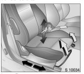
Seat adjustment: Seat height Seat position **Important:** Do not sit nearer than 10 inches (25 cm) from steering wheel. to permit safe airbag deployment.
