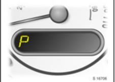
Display of the selected gear or mode with automatic transmission.
