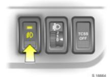
The front fog lamps can only be switched on when the ignition is on and the light switch is in position **>**€ or **ED**.
