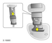
Insert latch plate into the slit on the belt webbing and insert detached connector latch plate in roof holder slot to the rear of the belt webbing.
