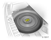
The temporary spare wheel is located in the luggage compartment and is secured with a screw-in retainer.
