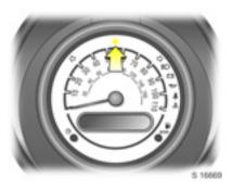
The theft-deterrent control indicator starts flashing after the key is turned to positions LOCK or ACC, or removed from the ignition switch.
