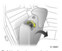
To fold outboard rear seatbacks separately \*\*, pull seatback release lever downwards, fold seatback forwards and down onto seat cushion.
