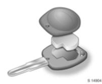
Remove screw on key cover and remove the transmitter.
