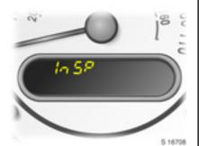
In the case of vehicles with fixed engine oil change and service intervals, InSP appears in the odometer display if the ignition is switched on when servicing is overdue: have the next service carried out within one week or 300 miles (500 km). Seek the assistance of a workshop.
