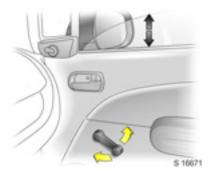
The door windows can be operated with the crank.
