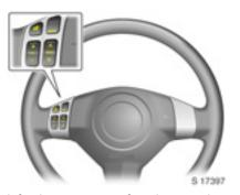
Infotainment system functions can be operated with the buttons mounted on the steering wheel.
