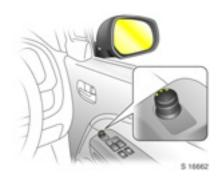
Adjust with the four-way switch in driver's door: Turn selector switch to left or right; four-way outer part of switch adjusts corresponding mirror.
