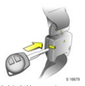
Unlatch detachable connector on centre rear seat belt by inserting the ignition key in the slot on the connector and allow the belt to retract.
