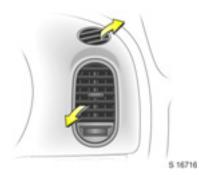
To open and close side air vents, turn horizontal knurled wheel to the left or right.
