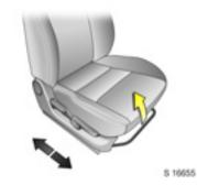
To adjust, pull the handle on the front seat, slide the seat and release the handle.
