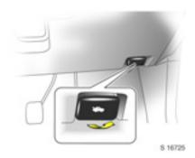
To open the bonnet, pull release lever - located on the driver's side of the vehicle, below the instrument panel.
