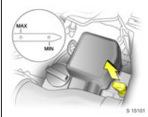
The illustrations show checking the engine oil in the K 10 B and K 12 B petrol engines and the diesel engines respectively.
