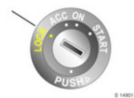
The system checks whether the vehicle may be started using the key that has been inserted. If the key is recognised as "authorised", the vehicle can be started. The check is carried out via a transponder housed in the key.
