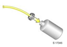
If you have a flat tyre: Shake sealant bottle, remove cap and screw filler hose on to bottle, to pierce inner cap.
