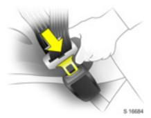
Insert the latch plate into the buckle. Seat belt buckles are designed such that latch plates cannot be inserted in the incorrect buckle.
