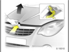
Locate the safety catch on the underside of the bonnet, push the catch to the left and lift the bonnet.
