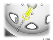
Unscrew valve cap from defective tyre and unscrew valve insert using supplied remover.
