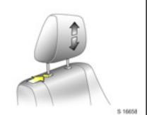
Adjusting head restraint height: Press catch, adjust height, then release
