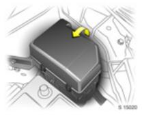
The fuse box is located next to the battery in the engine compartment.
