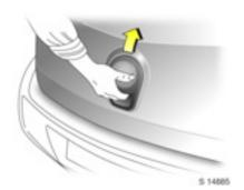
To unlock and open the tailgate: Press button ⓓ on remote control ※ or unlock with the key, operate button below the handle
