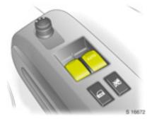
Operational with key in ignition switch position ON.
