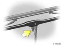
Lift wiper arm, press retaining clip towards wiper arm and detach wiper blade.
