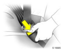
To remove the belt, press the red release button on the belt buckle; the belt will retract automatically.
