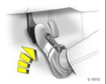
To manoeuvre the vehicle back and forth during attempts to park or in garage entrances, the creeping movement can be utilized by releasing the foot brake.
