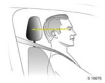
For maximum protection, the middle of the head restraint should be at eye level. If this is not possible for extremely tall persons, set to highest position, and set to lowest position for extremely small persons.
