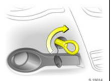
Screw in towing eye attachment clockwise until it is firmly in place. If necessary, use jack handle to tighten.
