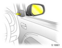
Adjust mirrors by swivelling lever in required direction.
