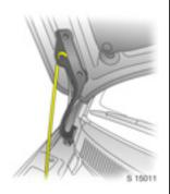
To hold the bonnet in the open position, disengage the support rod from its retaining clip and place in slot in underside of bonnet.
