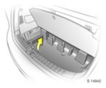
If necessary, the under floor storage compartment can be removed from the luggage compartment.
