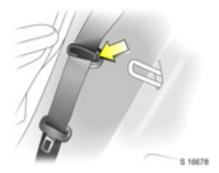
Route outboard rear seat belts, including the latch plates, through their respective belt holders (as illustrated), ensuring they are not twisted at any point.
