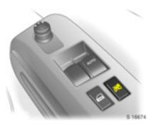
Press the 🗷 switch in driver's door to deactivate front passenger's door electric window operation when a child is occupying the seat.
