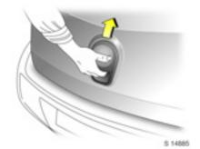
The tailgate can be opened by operating the button below the handle and lifting the tailgate.
