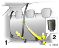
The centre rear seat belt position has a twin buckle arrangement. Engage the smaller latch plate (1) into the correct buckle, then pull the belt across and audibly engage into the buckle marked CENTER (2).
