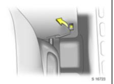
The tank flap is opened by pulling up the release lever located on the outboard side of the driver's seat.
