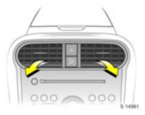
The air flow can be directed as desired by tilting the slats up, down and sideways using the central adjuster.
