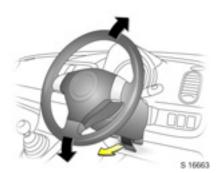
To adjust steering wheel \*, pull lever forwards, adjust height, push lever back and engage.
