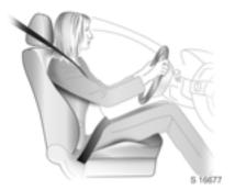
Adjust driver's seat such that, with the driver sitting upright, the steering wheel is held in the area of its upper spokes with the driver's arms slightly bent.
