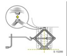
5. Position jack at the front or rear jacking point located nearest to the wheel concerned so that the jack claw spans the vertical base. Make sure it is properly positioned, ensuring the jacking bar fits securely into the jack head groove.
