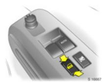
Use the central locking switch to lock or unlock the doors and tailgate from inside the vehicle.
