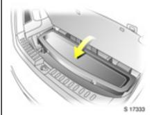
The luggage compartment cover can be stowed in the under floor storage compartment \*.
