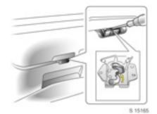
If the central locking system \* cannot be operated with the remote control, the tailgate can be opened from inside the vehicle.
