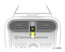
■ Switch on ignition; control indicator 2 flashes in the instrument panel then remains illuminated, to display the current status.
