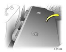
To fold rear bench seat \*, pull both outboard seatback release levers downwards simultaneously, fold seatback forwards and down onto seat cushion.
