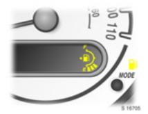
Indicates fuel level when the ignition is on (**F** indicates full, **E** indicates empty).
