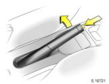
Always apply the parking brake firmly without actuating the release button. Apply as fully as possible on uphill or downhill inclines.
