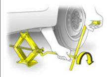
Rotate jack handle clockwise using the attached wheel bolt wrench to raise vehicle.
