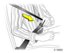
Pull the belt out evenly from the retractor and guide it over the shoulder, making certain that it is not twisted at any point. The belt must not rest against your neck or arm.
