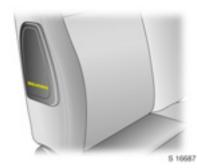
The side airbags are identified by the words **SRS AIRBAG** on the outboard side of the front seatbacks and on the B-pillar.
