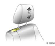
To adjust head restraint height, press catch, adjust height to suit then release the catch.
