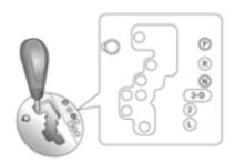
Park position. Front wheels locked. Only engage when the vehicle is stationary and the parking brake is applied. "P" appears in the transmission
