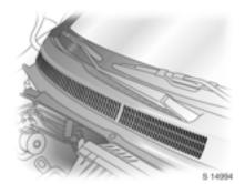
The air intakes in front of the windscreen in the engine compartment must be kept clear to allow air intake. Remove any leaves, dirt or snow.
