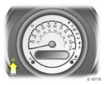
If there is a problem with the automatic transmission, control indicator **\$\Pi\$** flashes. The transmission no longer shifts automatically.
