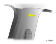
The curtain airbag system is identified by the words **SRS AIRBAG** on the roof frame.
