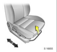
Longitudinal seat adjustment: Pull handle, slide seat, release handle Seats \$⇒ 3-2.
