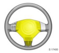
The front airbag system is identified by the words **AIRBAG** and **SRS AIRBAG** on the steering wheel and above the glove box respectively.
