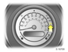
Indicates when the engine oil and oil filter require changing. Based on driving conditions, the interval at which an oil change will be indicated can vary considerably.
