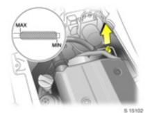
Top up if the engine oil level has dropped to the "add oil" lower mark (**MIN** mark).
