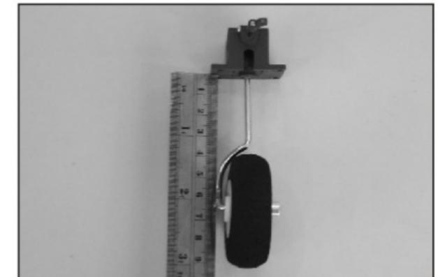
4. Same way to assemble the nose gear and adjust the wire at 65mm (2-1/2") in length.
