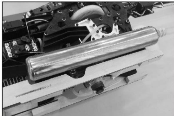
21. Install the muffler and check if muffler contacts the wood mount. You may need to trim the wood mount. (photos shown is OS91 with Zimmerm muffler) The kits comes with muffler extension that you may use. Check if the throttle lever contacts the muffler if you use the extension. Trim the contact area if necessary.
