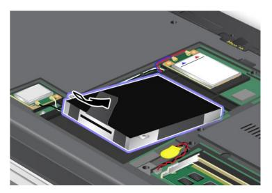
8. Slide the hard disk drive firmly into the connector 1, and then reinstall the screws 2.
