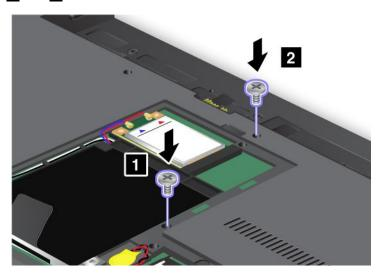
5. Attach the cover 1, pivot it downwards, and then tighten the screws 2.
