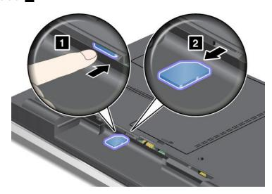
5. Insert the SIM card firmly into the slot.
