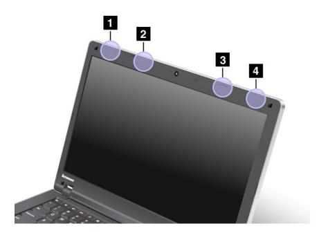
Wireless LAN and WiMAX combo antenna (Auxiliary)
