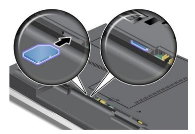
Note: Make sure that you insert the SIM card all the way into the slot.
