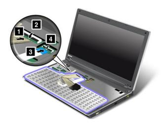
2. Insert the keyboard. Make sure that the rear edges of the keyboard are under the frame, as shown by the arrows.
