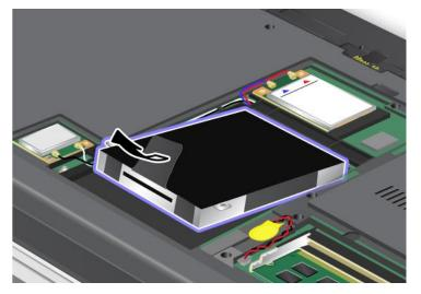
7. Place the new hard disk drive from the lower side as shown in the picture.
