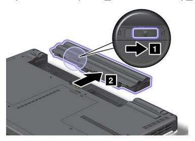
4. Insert a fully charged battery until it clicks into place 1 as shown in the drawing, and then slide the battery latch to the locked position 2.
