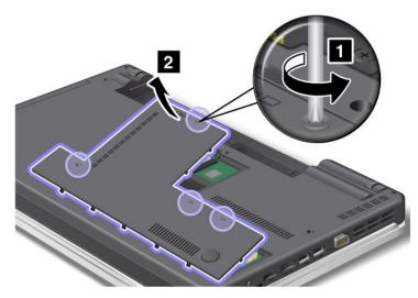
5. Remove the screws 1, and then slide the hard disk drive towards the front of the system 2.
