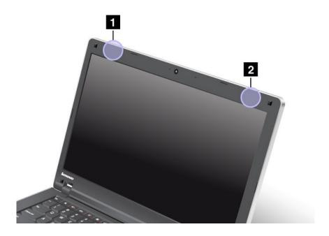
1 Wireless LAN and WiMAX combo antenna and Wireless WAN antenna (Auxiliary)
