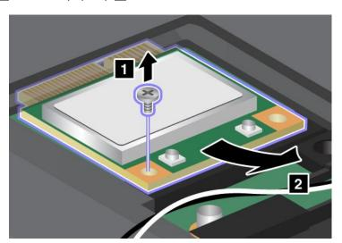
7. Align the contact edge of the new PCI Express Mini Card with the corresponding socket 1. Pivot the card until you can snap it into place. Secure the card with the screw 2.
