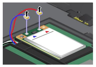
6. Remove the screw 1. The card pops up 2. Remove the card.
