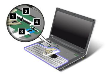
2. Insert the keyboard. Make sure that the rear edges of the keyboard are under the frame, as shown by the arrows.
