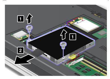
6. Remove the hard disk drive by lifting its upper side.
