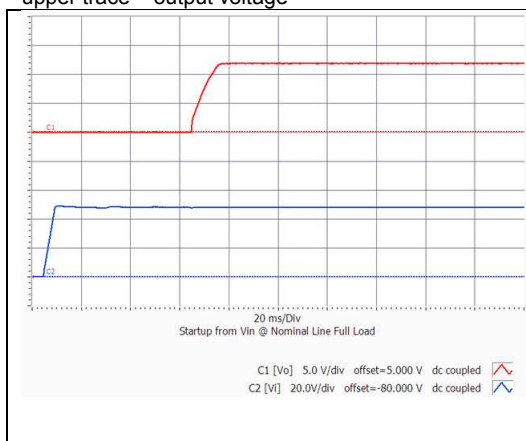
iQE4W011A120V-001 Typical startup characteristic from input voltage application at full load. Upper trace - output voltage, lower trace -input voltage
