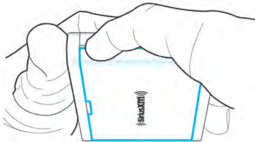
2. Orient the battery as shown and install it into the battery compartment.
