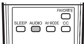
You can change MTS as shown below to match the television broadcast signal. Press **AUDIO** to toggle between audio modes.
