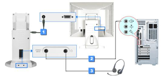
Connect the power cord of the multimedia stand to the multimedia stand power port on the back of the monitor.
