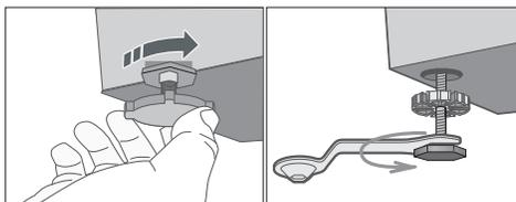
6. Level your Washer by turning the leveling legs in or out as necessary by hand or wrench included with your Washer.
