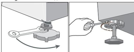
7. If you install your washer on soft floor, you should place the rubber cup under adjustable leg. Before put rubber cup, please remove film for double-side tape attached on rubber cup.
