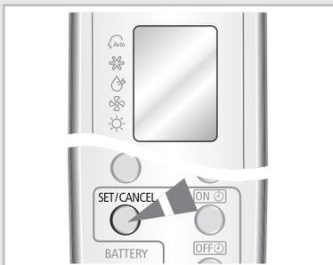
**You can set the On Timer to turn on the air conditioner automatically at the appointed time. You can set the time from 1 hour to 24 hours.**
