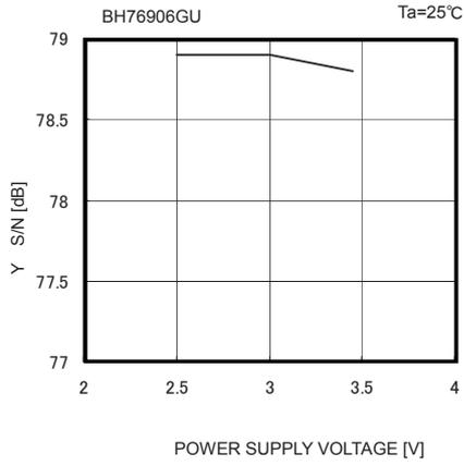
Fig. 47 Y S/N vs Supply Voltage
