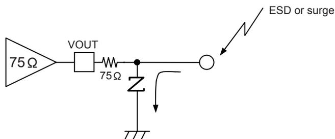
Fig.59 Using Externally Attached Varistor
