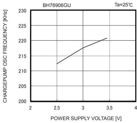
Fig. 39 Charge Pump Oscillation Frequency vs Supply Voltage
