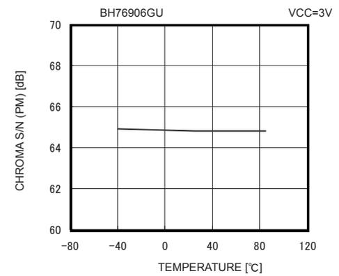
Fig. 52 C PM S/N vs Ambient Temperature
