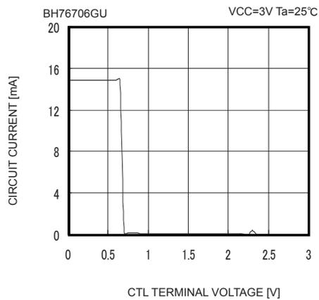
Fig. 56 Control Pin Characteristic
