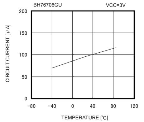
Fig. 21 GND Mode Circuit Current vs Ambient Temperature
