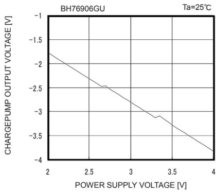
Fig. 41 Charge Pump Output Voltage vs Supply Voltage
