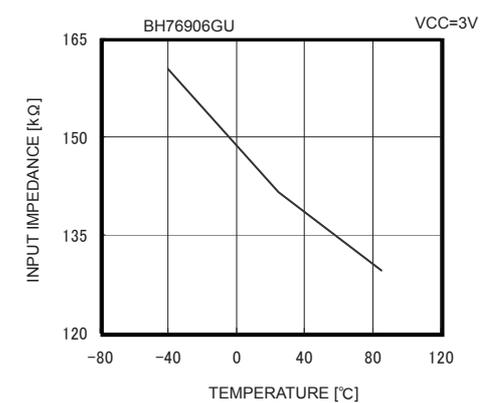
Fig. 54 Input Impedance vs Ambient Temperature
