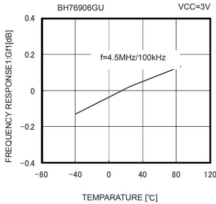
Fig. 29 Frequency Characteristic 1 vs Ambient Temperature
