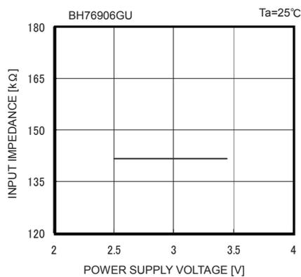
Fig. 53 Input Impedance vs Supply Voltage
