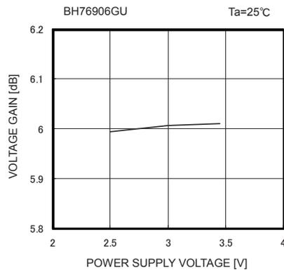
Fig. 26 Voltage Gain vs Supply Voltage
