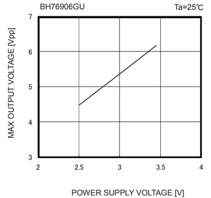
Fig. 36 Max. Output Level vs Supply Voltage
