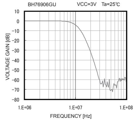
Fig. 24 Frequency Characteristic
