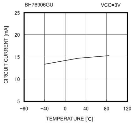
Fig. 17 Circuit Current vs Ambient Temperature
