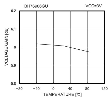
Fig. 27 Voltage Gain vs Ambient Temperature
