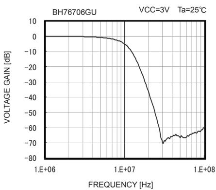
Fig. 25 Frequency Characteristic
