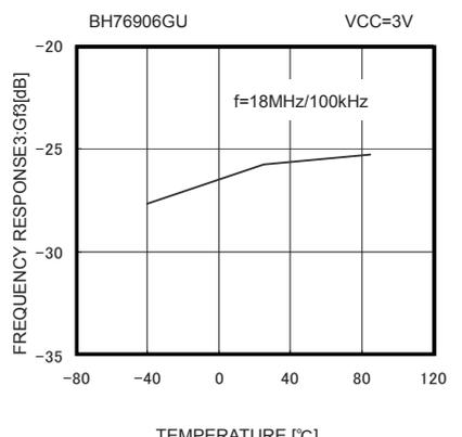
Fig. 33 Frequency Characteristic 3 vs Ambient Temperature
