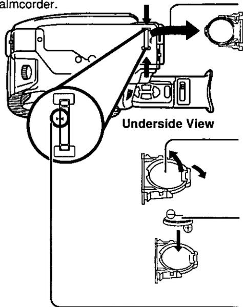
**1** While pinching the stopper tabs, pull the Battery Tray out of the Battery Compartment.
