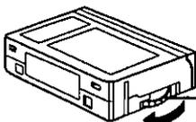
**1** Turn the Tape Wheel on the **VHS** cassette in the direction of the arrow to take up any slack.
