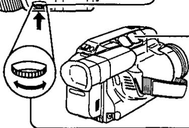
**2** Press and hold the "T" side of the **POWER ZOOM** switch until the lens is zoomed in all the way (subject at maximum size).
