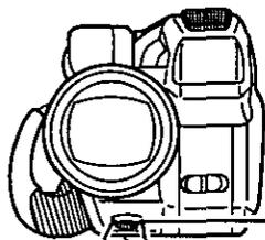
**1** Press **MANUAL FOCUS** so that "MF" (Manual Focus) appears in the EVF.
