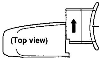
**2** Slide the eyepiece in the direction of the arrow. (DO NOT TWIST)
