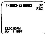
**2** Press DISPLAY twice to change the display to date only. Press once or twice more to remove the date/time display.
