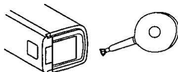
**3** Remove any lint or dust particles with a blower, available at photography stores. Do not touch lenses with fingers. Then, replace the eyepiece.
