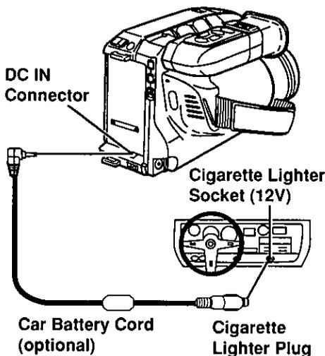
**1** Connect a PV-C16 Car Battery Cord (optional) to DC IN on the Palmcorder.
