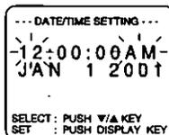
Press or hold down **UP ▲** or **DOWN ▼** to select hour, then press **DISPLAY** to fix.
