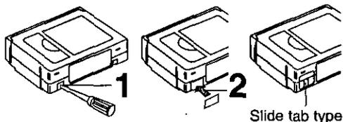
**1** To prevent accidental erasing, **break off tab** with screwdriver.
