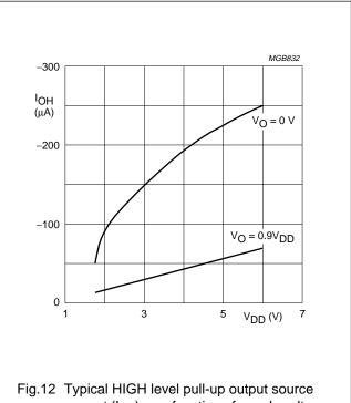
current (I<sub>OH</sub>) as a function of supply voltage  $(V_{DD}).$
