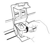
**5** Take the ink cartridge out of its packaging and remove the protective strip. Be careful not to touch the nozzles and the contacts.
