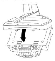
7 Insert the chip card "Plug 'n Print" with the contacts facing up into the slot under the control panel and confirm with OK. Remove the cartridge and repeat the process for the second cartridge.
