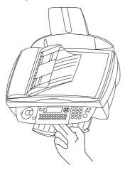
**6** Remove the protective tapes from the cartridge holder and close the machine.
