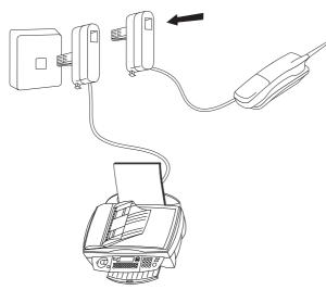
Connecting additional devices to the same socket ensures you the optimal functionality of your active fax switch (e.g. call transfer). Your fax machine can control the additional devices.
