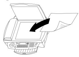
**3** Align it with back left corner of the scanner (marked with arrows).
