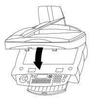
**9** Insert the chip card "Plug 'n Print" with the contacts facing up into the slot below the control panel to update the cartridge information. Press **OK**.
