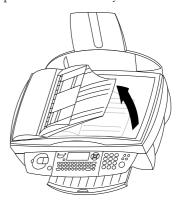
**5** Open the machine by pulling the lever under the control panel.
