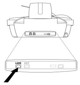
Next connect the telephone plug to the line socket on the wall.
