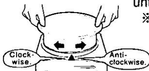
※ Insufficient tightening causes steam to escape, thus preventing proper steaming.
